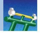
The bar model is pinned. Observe the fundamentals of pinning (from thick to thin!) and that the connectors must be provided with at least 3 mm casting channels.
